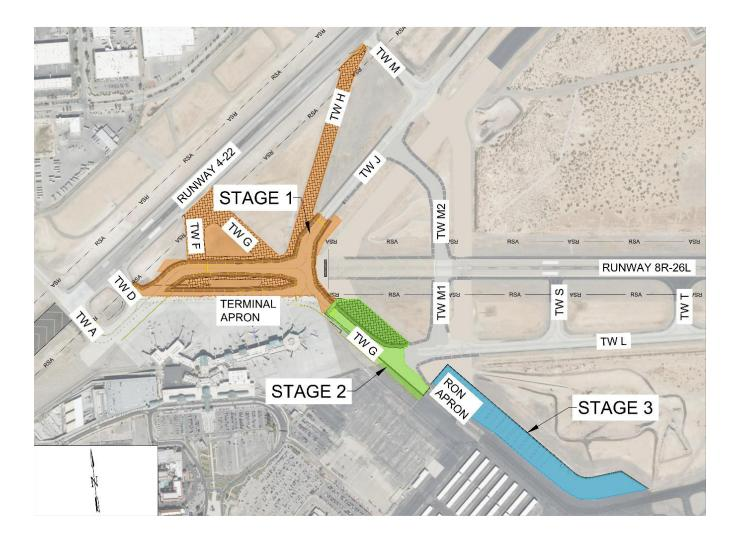
The Five Node Intersection Remediation project improvements include rehabilitation and reconfiguration of the parallel taxiway, connectors, and terminal apron taxi lane near the 8R Runway end. Other improvements include associated airfield lighting, grading, and drainage in the project area.
