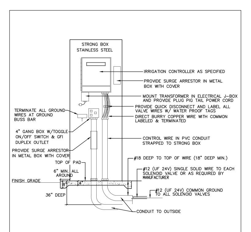
NOTES: 1. GROUND CABINET WITH #10 GAUGE OR HEAVIER STRANDED COPPER WIRE TO GROUNDING ROD AS PER MANUFACTURER'S SPECIFICATIONS.
